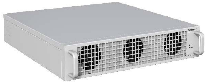
400V Ultra SVG 100 kVar (Rack) Size: 500x520x100mm (WxDxH)
